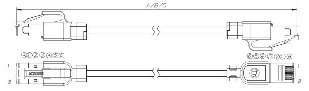
Cable printing: MICROLINK CAT.6(A) S/FTP 4PR 26AWG LSZH PATCH CABLE FT4 D 0A7I001-1
